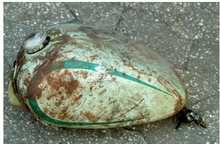
Unfortunately we find with historic vehicles not only rust inside the tank, we also find from time to time rust perforated tanks that allow fuel leakage. The TAPOX 2-part internal protection is very resistant to fuel, but is designed to be very thin and so does not close fine holes or cracks in perforated tanks.
